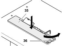
5. Turn the countersunk screw (36) counter-clockwise against the stop.
